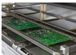
Grip conveyor for extremely thin PCBs or flexfoils
