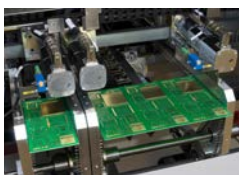
Multi track conveyor for variable PCB width
