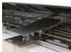
Retractable nozzle sheets for quick maintenance
