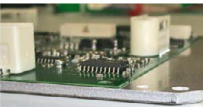
SOIC & Plastic SMT on Aluminium Carrier
