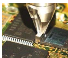
Small footprint of Flip Chip lens: 0.6 \text{ mm} \times 4.0 \text{ mm}
