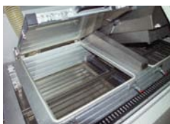
Flexible preheating concept: medium and short-wave emitters
