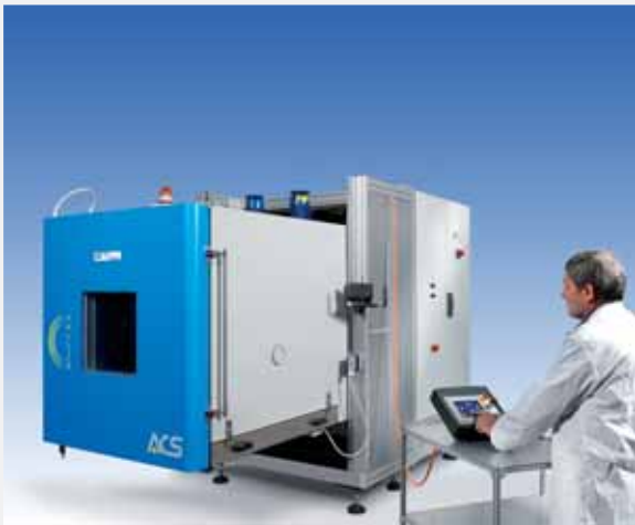
Test cabinet movement can be set by a detachable touch-screen control panel.
