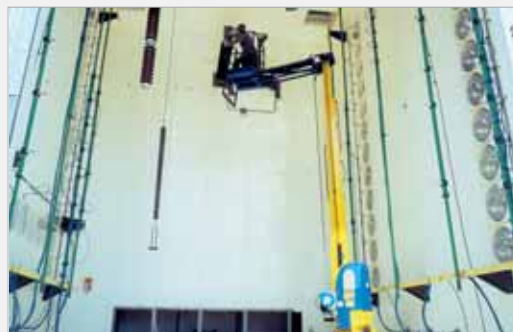
Test chamber for accelerated-aging of high voltage isolators: temperature, humidity, sun light, salt spray. Useful capacity: more than 700 m 3 (courtesy EDF France)
