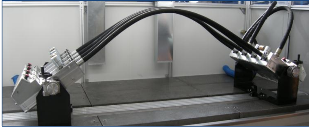
View of the test chamber with 4 hoses connected
